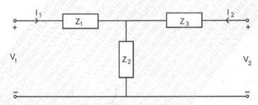
3 (A) Determine Thevenin's equivalent network for the Fig. shown.
